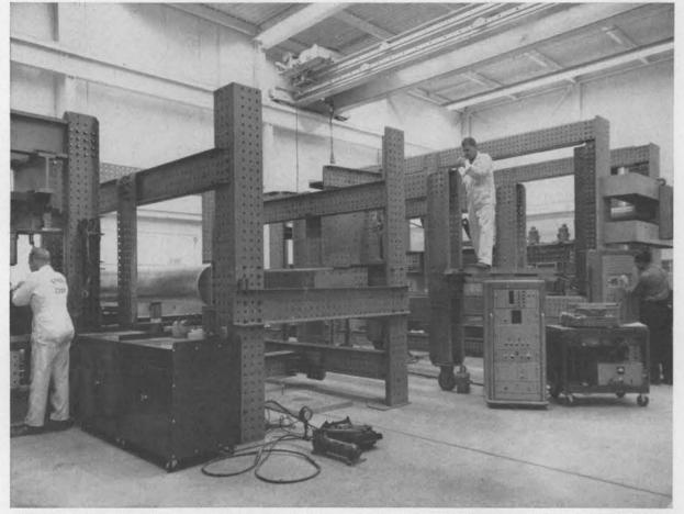
NO GIANT ERECTOR SET, this static test facility is used to apply stresses and strains on weapons components in Bldg. 864 to simulate conditions which may be encountered in actual use. Shown
